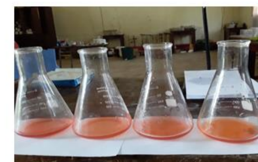
Fig: Shubiri solution after titration with mbilimbi solution (Acidic). It gave same results with Hydrochloric Acid |
