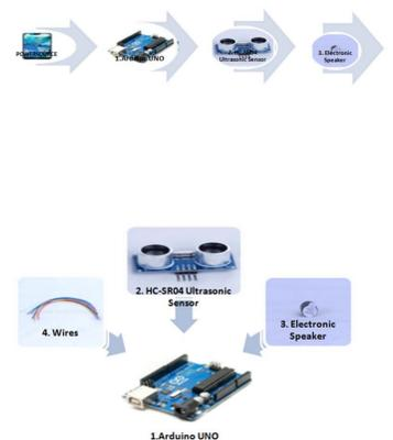
When an object is detected in the distance of 0 to 1 meter (100 cm), the electronic speaker is triggered and continuous sound. But, when an object is detected in the distance of 0 to 1.02 meter (102 cm) the device can either beep sounds. If it is 1.02 meter (102 cm) and above, it doesn't produce any sound.
