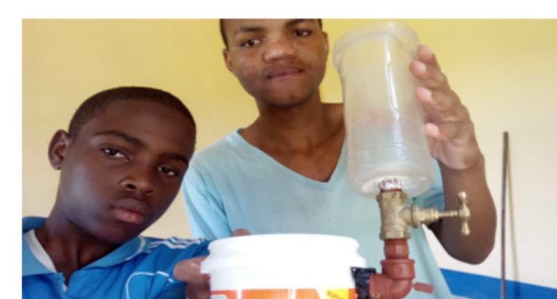
Picture showing busy task Making mixing tank • First, two holes at the base walls of small bucket was made to make glue outlets • Second, petrol tank was fixed at the mixing tank through small hole at the upper side of mixing tank. • Third, the buoy outlet was joined to the mixing tank. • Fourth, the three finished tanks systems were fixed together making complete glue production tanks systems.
